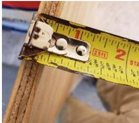
Photo showing dimensions of decking nail used (min. diameter 0.113 in. and min. length 2 3/8 in)
